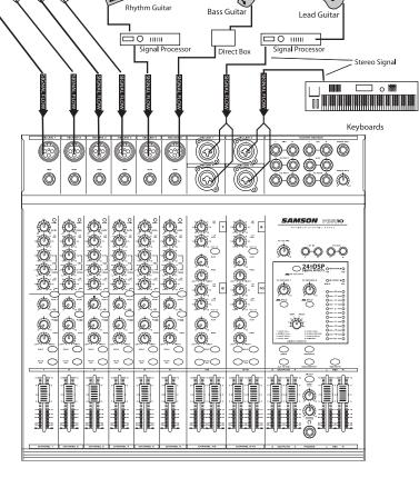
**OFF**". Translated, this means that when turning on your system, you should always turn your power amplifiers or powered monitors on LAST, and when turning your system off, turn your power amps off FIRST. This helps avoid any loud pops caused by rush current at power up, which can sometimes damage loudspeakers.
